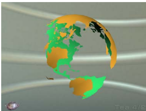
Fig 58 The same model with the ZOffset=10 User Defined Property removed. Note that the orange under sides of the continents that are on the back side of the globe are rendered on top of the front facing continents.
